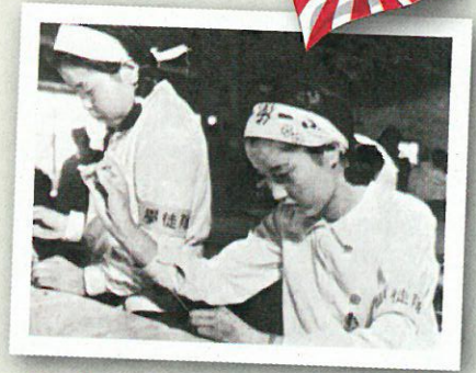
ABOVE Delicate and demanding work — teenage Japanese girls hard at work stitching the envelope for another balloon. The glue used for pasting the envelope was derived from the "devil's tongue" root, and was frequently eaten.
